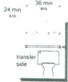
Figure 604.5.2 Rear Wall Grab Bar at Water Closets
