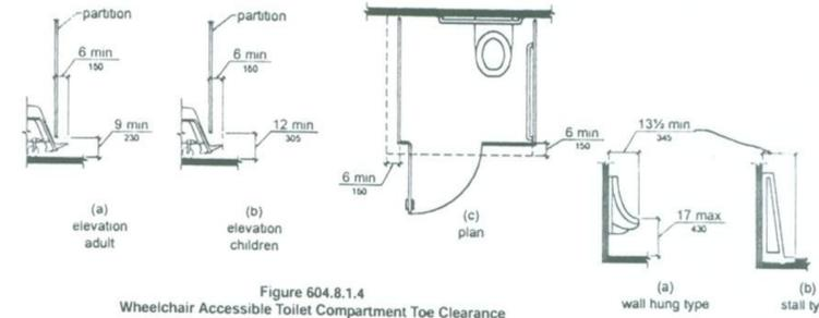
Figure 604.8.1.4 Wheelchair Accessible Toilet Compartment Toe Clearance
