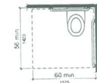
Figure 604.3.1 Size of Clearance at Water Closets
