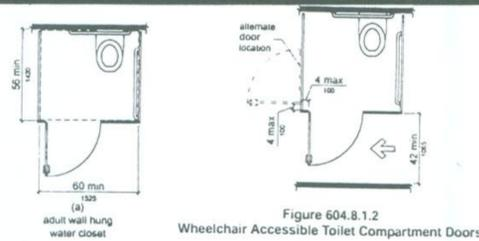
Figure 604.8.1.1 Size of Wheelchair Accessible Toilet Compartment
