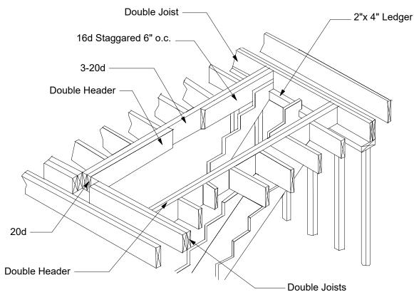
JOISTS PERPENDICULAR TO STAIRS
