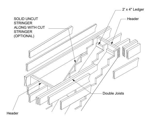
JOIST PARALLEL TO STAIRS **FLOOR OPENINGS**
