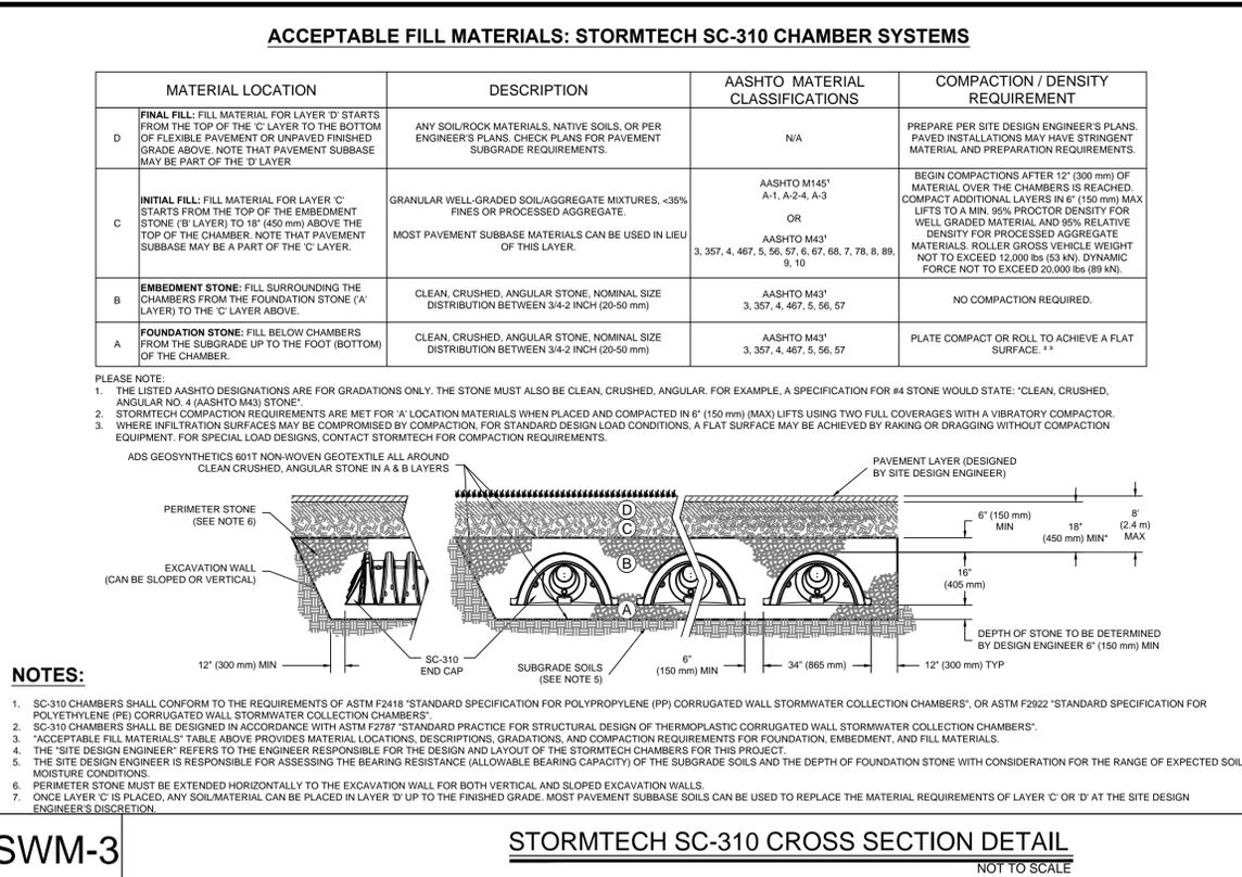
**SWM-3** **STORMTECH SC-310 CROSS SECTION DETAIL**
