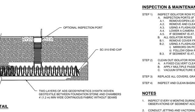
**SWM-5** **STORMTECH FLUSING/INSPECTION PORT DETAIL**
