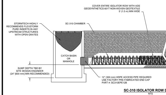
**SWM-4** **STORMTECH SC-310 CHAMBER DETENTION ISOLATOR ROW DETAIL**
