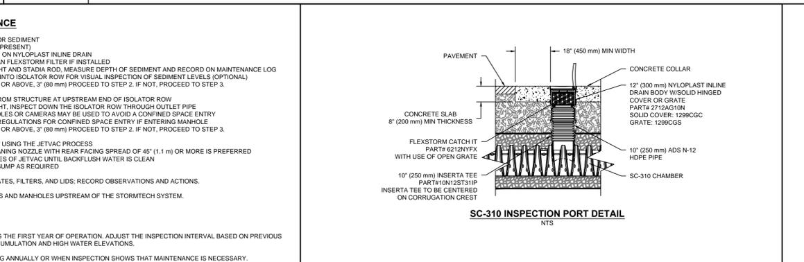
**SWM-5** **STORMTECH FLUSING/INSPECTION PORT DETAIL**
