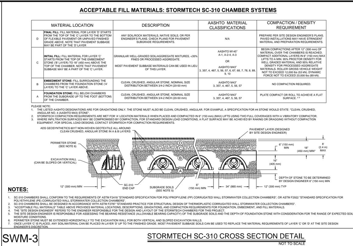
**SWM-3** **STORMTECH SC-310 CROSS SECTION DETAIL**
